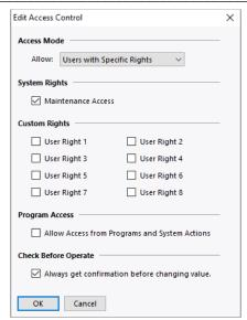
If the Program Access box is checked, remote access to write to the data points is enabled without any additional security checks. Unchecked write-protects the values.
