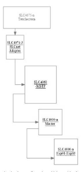
• This is the simplest configuration which provides for a single boiler with up to 32 relay steps.
